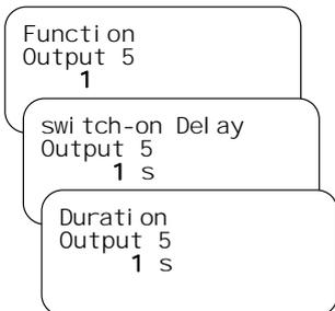
With regard to the outputs, using the parameterisation – software it is possible to select whether the relay should open or close when a signal / event is received (closed-circuit/open-circuit principles).
