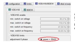
For systems with more than 30 kVA, the corresponding value must be activated in the parameterisation (figured left). The voltage monitoring then takes place both at the star-point voltage and at the external connector voltage.
