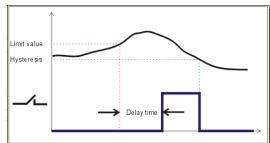
Each switching point can be assigned to a relay output (see chap. 11.1 - Digital Outputs) The output relay then switches according to the parameterisation when the respective measured value is exceeded or undershot. No messages are displayed.
