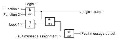
All logic and timer functions can be assigned to the fault message groups and to the collective fault. The available blocking functions are also available for all logic and timer functions. Each input function is invertible.
