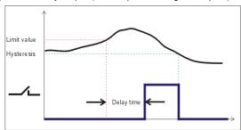
The output relay then switches according to the parameterisation when the respective measured value is exceeded or undershot. No messages are displayed.
