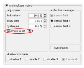
(enter Button) while main screen is displayed. The manual reset works edge-controlled and resets all limit messages for 1 s. If limit value messages are still pending, they are again indicated with the end of the reset time.
