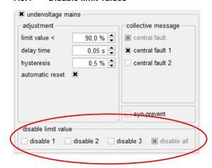
Individual or all limit value messages can be deactivated by means of the parameterisable digital inputs (see chap. 11.1). Up to 3 blocking functions can be assigned to each limit value. The global lock function 'disable all' always deactivates all active limit messages. If the input is set, the corresponding limit value messages are suppressed. The following lock functions are available:
