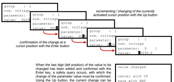
Actuating the Enter button (ENT), the entry of the parameter value is accepted and stored in the flash memory of the SYN-8. The value is valid immediately after confirmation.
