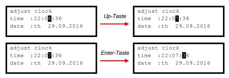
The procedure described above must be repeated for all positions of the time and date input.
