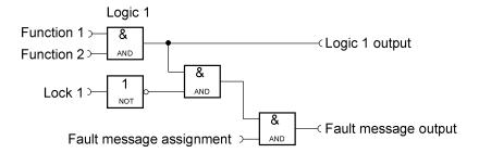
All logic and timer functions can be assigned to the fault message groups and to the collective fault. The available blocking functions are also available for all logic and timer functions. Each input function is invertible.
